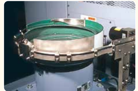
● Parts feeder This is a bucket type stocker suited to small workpieces that do not take up much space. The part feeder can be directly linked to a conveyor.
