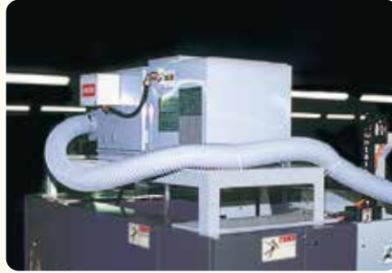
● Oil mist collector Collection of oil mist helps to keep the environment clean.
