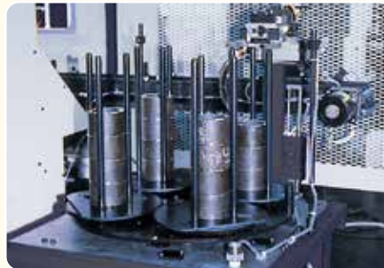
● Station stocker Multi-level stocker that allows a flexible response to changes in workpiece diameter.
