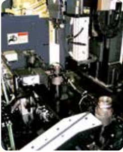
● External measurement Dimensional error is fed back to the machine to maintain high-quality dimensional accuracy.
