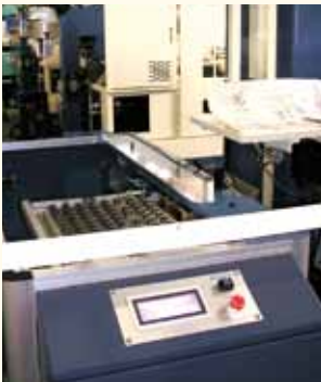
● Tray Changer By stacking per pallet, scratches on parts are prevented because of better stacking resulting to an efficient form of delivery system.
