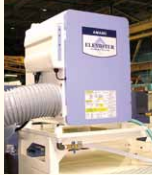
● Oil mist collector Oil mist collection facilities a clean production environment.
